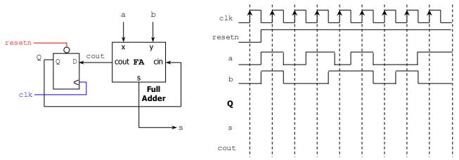
Complete the timing diagram of the circuit shown below. Get the excitation equation for Q. (7 pts)
