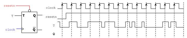
b) Complete the timing diagram of the circuits shown below: (6 pts)
